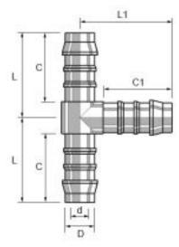
C: 16 mm C1: 16 mm D: 4 mm L: 19 mm L1: 20.5 mm
